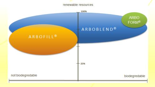
ARBOFORM® is based on the nearly unlimited, abundant raw material LIGNIN (by-product from the pulp industry), adding natural waxes, resins and fibers. Fully bio-based, it is also widely known as LIQUID WOOD.
