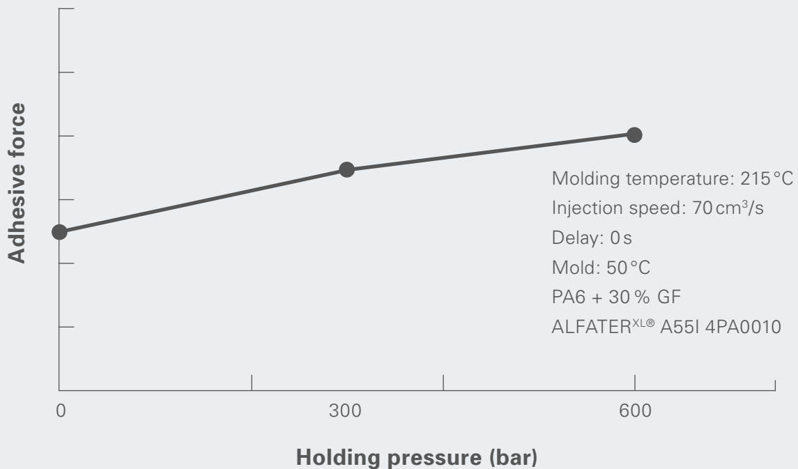
Figure 7: Influence of holding pressure of ALFATER XL ® 4PA0010 on adhesion to PA.
